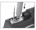
Place the handpiece on top of the new cartridge and press down slightly.
