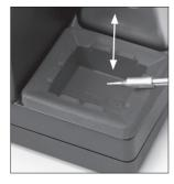
Tapping:Tap gently to remove excesssolder.
